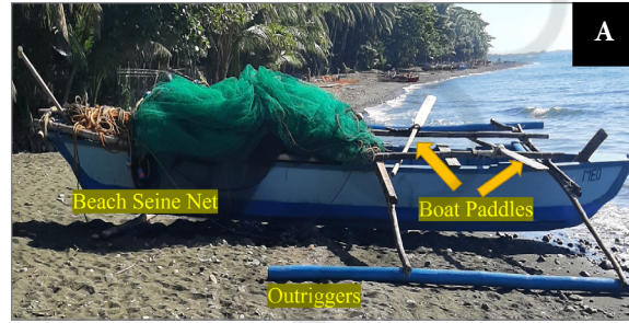
Figure 2A. A typical beach seine in Brgy. Damilisan, Miagao, Iloilo with labeled parts.
